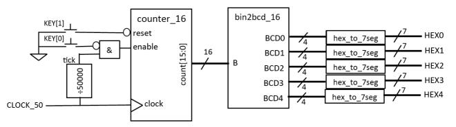
Modify your circuit to implement this and test the new circuit on the DE1 board.
